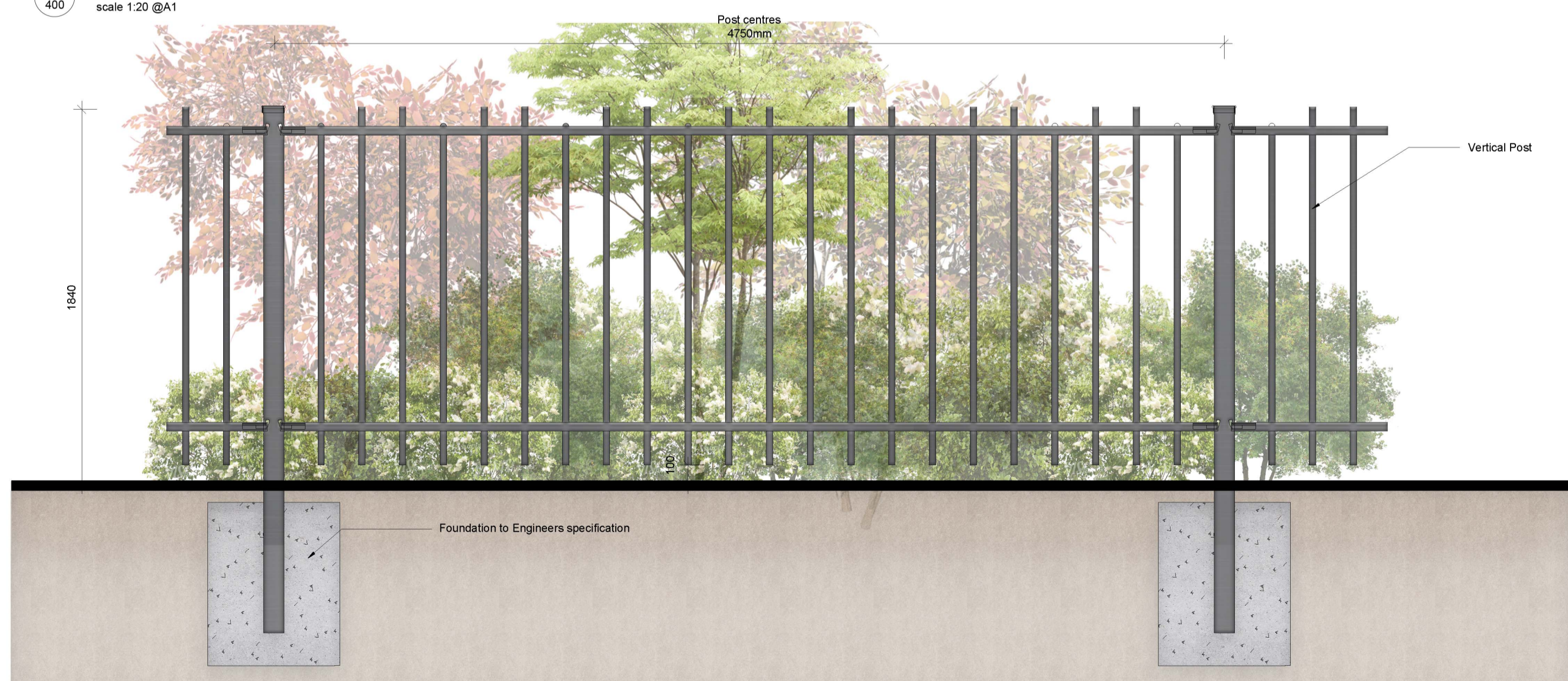
6 Proposed Steel Fence- elevation scale 1:20 @A1
