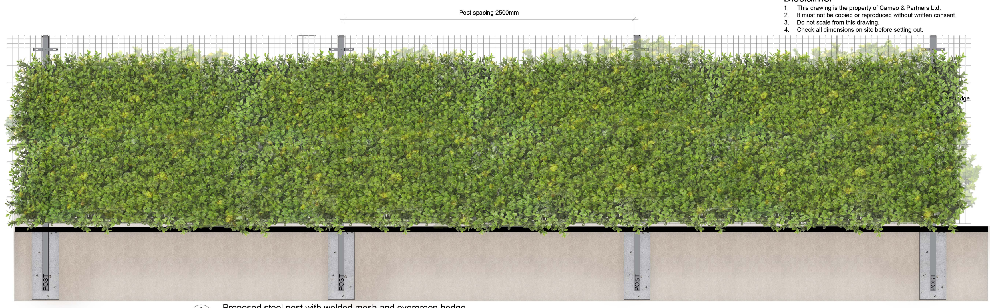
2 Proposed steel post with welded mesh and evergreen hedge scale 1:20 @A1
